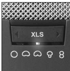
Fig. 1: Polar pattern selector.
