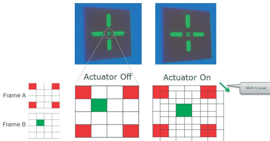
Figure 4. Working principle of the Optical Actuator
