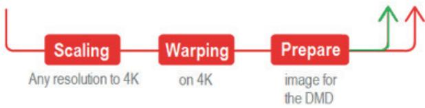
Figure 1. Conventional sequential processing steps in a projector
