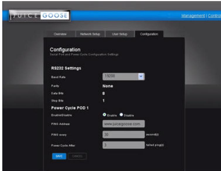
You can also assign a new IP or control the device via RS232 commands (see page 13 and 14 for the list of commands), this will require a special cable (detailed drawing on page 13).
