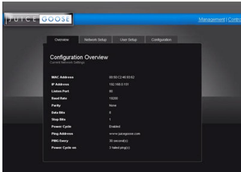
The Overview Tab displays the current settings of the unit and the MAC address. This page is useful for retrieving all the information you may need to set up the iP15 on your network. If you have DHCP enabled, the IP address your router/DHCP server assigned can be viewed here.
