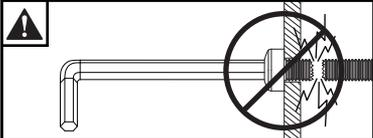
ENG Do not overtighten screws.
