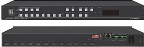
VS84H2 is a highperformance 8x4 matrix switcher for 4K@60Hz (4:4:4) HDR signals and digital audio routing. It reclocks and equalizes the signals and can route any one of 8 HDMI, HDCPcompliant sources (selectable) to any or all outputs simultaneously. VS84H2 offers unmatched audio flexibility where any embedded digital audio input can be routed to any digital output in addition to four ARC sources to produce an equivalent 12x8 audio matrix
