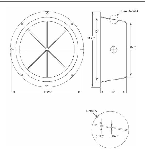
This enclosure will not accept a driver with a magnet weight greater than 10 oz. and a mounted transformer with taps greater than 8-watts.
