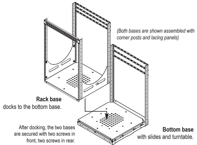
Removable rack base allows shop wiring of equipment.
