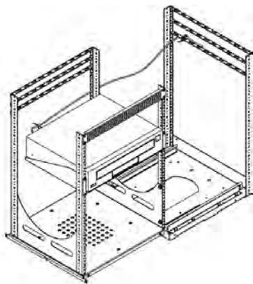
Rack in 90° position with cabling tied off.
