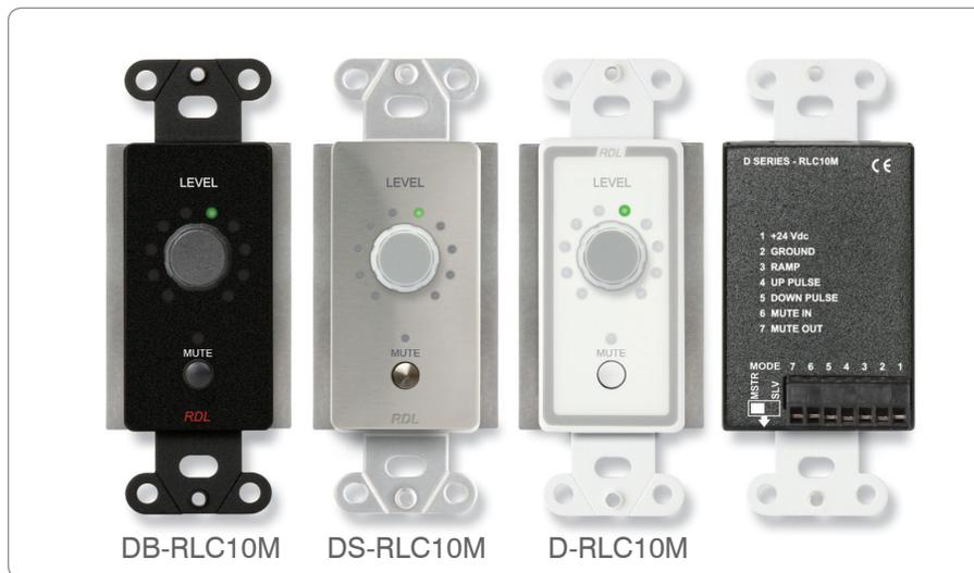
The **D SERIES-RLC10M** is a rotary remote level control with pushbutton muting that provides user adjustment at single or multiple locations. Optical encoder technology allows continuous knob rotation with a comfortable adjustment rate and long-term trouble-free and noise-free operation. These controls directly connect to any RDL VCA and OEM equipment with 0 to 10 Vdc ramp inputs.
