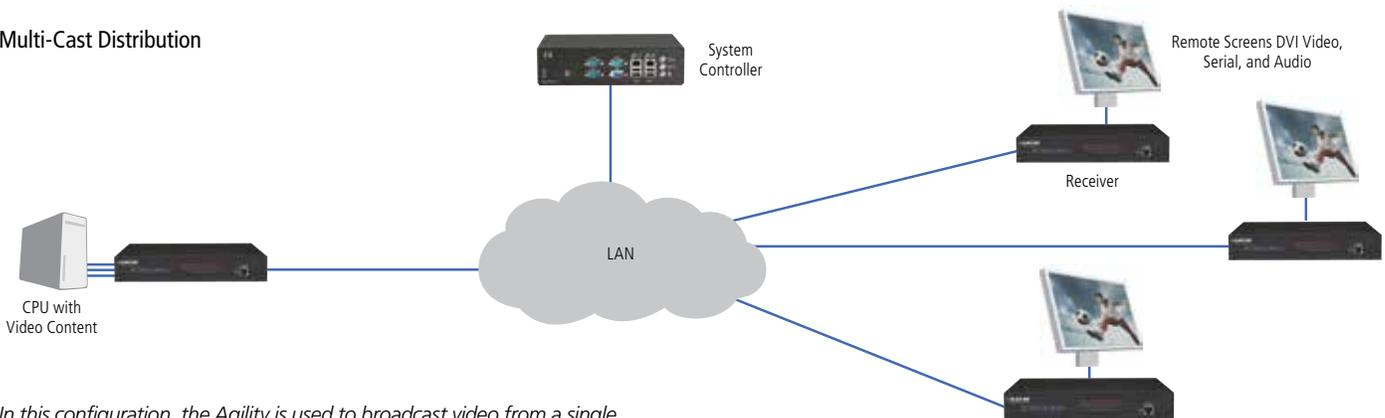
In this configuration, the Agility is used to broadcast video from a single CPU to remote screens.
