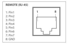
The selectable functions for PIN 1~ PIN 6 are as follows:
