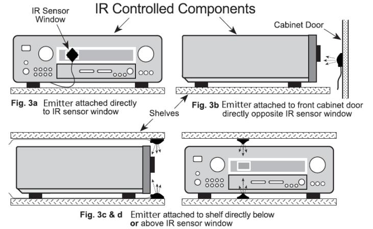
CAUTION: Cabinet door locations (Fig. 3b) will usually result in interruption of the IR control signals to the components when the door is open.
