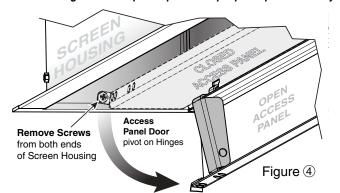
③ Press up on access panel and pull toward the front of the screen housing to disengage hinges and remove access panel.
