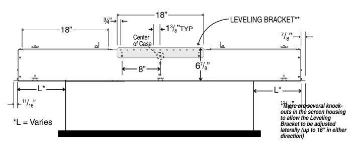
For ceiling cutout subtract 11/2" from case length and width (measured from outer edge of flanges).
