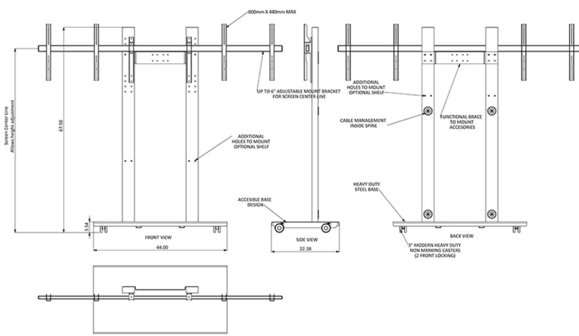
The **SYZ80-D** mobile interactive stand for dual TV's and interactive touch screen displays supports up to 2x 70" screens with a total weight capability of 250 lbs. Its unique modern design is ideal for corporate and educational environments. Both columns attached by a brace provide strength and support to the interactive board mounted. These columns feature grommets both on the top and bottom for passing cables inside the unit, leaving it with a very clean controlled appearance.
