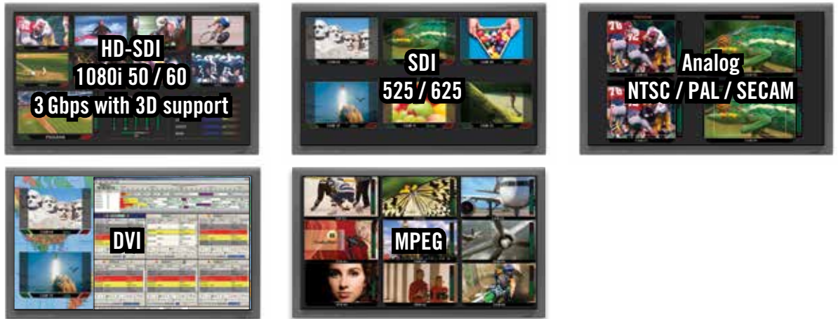
Auto-sensing inputs allow multiple source formats to be combined. DVI and MPEG are input via external options.
