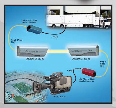
Using media converters, the broadcaster converted the HD-SDI signal from the HD camera to single-mode fiber-optic cable, which interfaced directly to a Canobeam DT-150 HD. The HD-SDI signal was received by a second Canobeam DT-150 HD, relayed via single-mode fiber and converted back to coaxial cable via a media converter, and then received by the HD broadcast truck.
