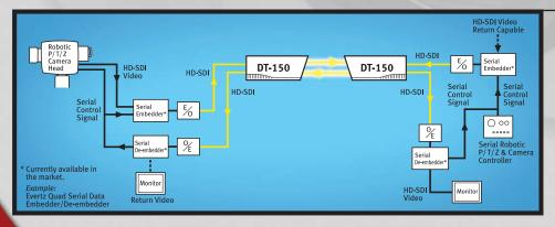
Using technology such as Evertz's Quad Serial Data Embedders and De-Embedders and a pair of Canobeam DT-150 HD video transceivers, the network is able to transmit HD-SDI video signals from the PTZ camera to their control room while simultaneously transmitting the required control signals back to the robotic PTZ head and its camera.
