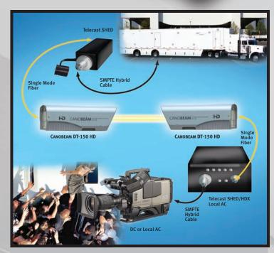
By using Telecast Fiber Systems' SHED (SMPTE Hybrid Elimination Device) or similar technology on either end of the connection, a pair of Canobeam DT-150 HD units can provide not only bidirectional HD-SDI video with embedded audio, but also bidirectional camera control signals, return video, tallys, and IFB.
