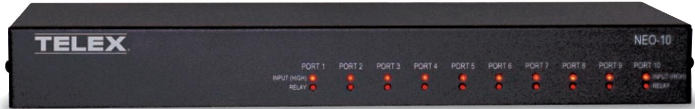
The NEO-10 is a network-based input/output device that has 10 DPDT relays and 10 inputs for monitoring external events. Anytime a relay or input changes, the NEO-10 sends out a message across the network, allowing all console users on the system to see status updates in real time. Actual control of the NEO-10 is accomplished by a TCP/IP socket connection from the controlling console.
