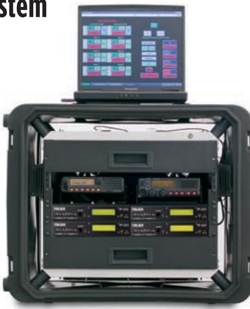
The idea behind V.I.P.E.R. is a fairly simple: use our innovative IP dispatch technologies to create complete self contained dispatch networks that are easy to deploy in emergency situations, providing an effective communications interoperability solution. Radio system interoperability is achieved instantly through simple crosspatches on the console. The IP-based system increases the reliability of the system, and makes it easy to add additional radios or dispatch positions on scene.
